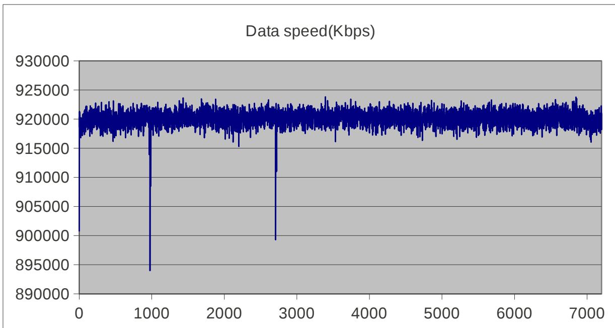
The drops on the 2 hour TCP traffic graph are caused by other processes running on the PC
