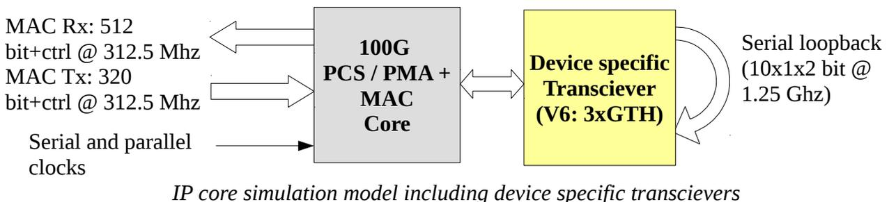
In this case the only generated clock signal is the reference clock for the GTH serdeses, the Rx/Tx MAC clock is derived from the GTH parallel clock:
