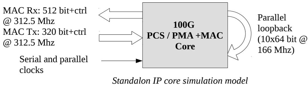
In this case the clock signals are generated from the testbench by previously defined constraints:
