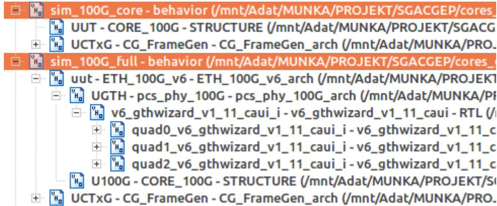
*Behavioural simulation testbenches for the 100G core*
