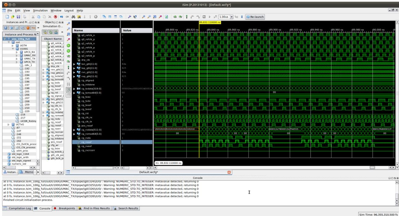
Simulating the IP core in iSim
