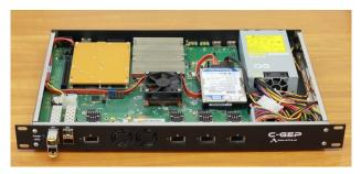
The main purpose is to provide means for handling 1, 10, 40, and 100 Gbit/s Ethernet traffic in a flexible manner.
